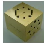
Fabricated OMT(Brass with gold-plating)
